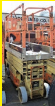
JLG 2630ES SN:200134281 electric powered, equipped with 26ft. Platform height, slide out deck, 500lb lift capacity.
