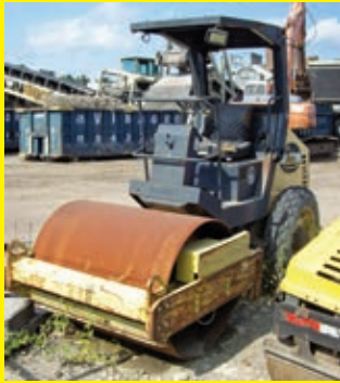
BOMAG BW124DH-3 SN:902581271102 powered by Deutz diesel engine, equipped with OROPS, 47in. Smooth drum, vibratory drum, drum drive.
