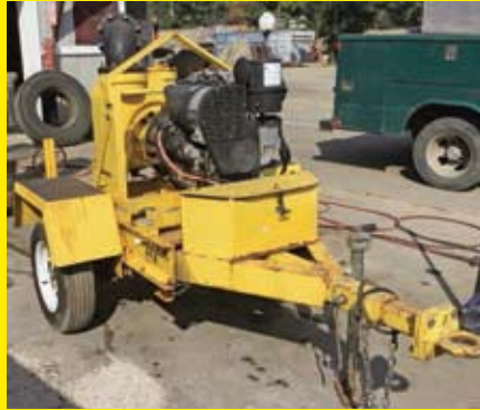
WACKER PT6 VN:203017 Lombardi diesel engine, trailer mounted.
