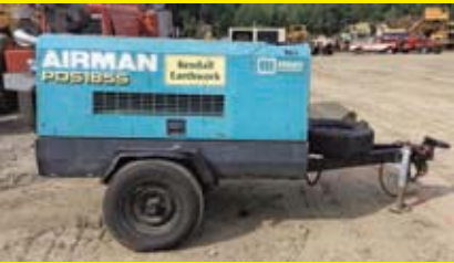
AIRMAN PDS185S diesel engine, 185CFM, trailer mounted.
