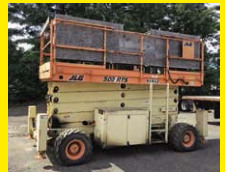
JLG 500RTS 4x4, diesel engine, 50ft. Platform height, slide out deck, (4) outriggers, rough terrain tires.
