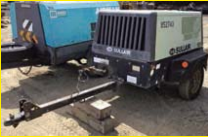
SULLAIR 185CFM diesel engine, 185CFM, trailer mounted.
