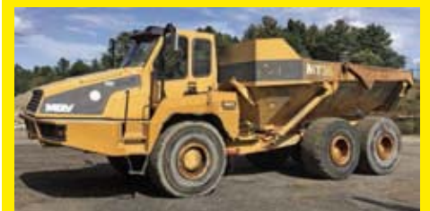
MOXY MT36 SN:410141 6x6, Scandia diesel engine, 400hp, Cab, 6 speed transmission, 36 ton capacity, tailgate, 26.5R25 rubber.
