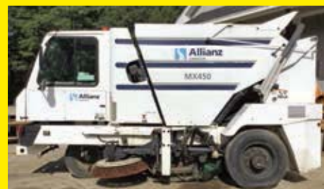
ALLIANZ JOHNSON VN:172064 diesel engine, sweeper body, dual wheel single axle.
