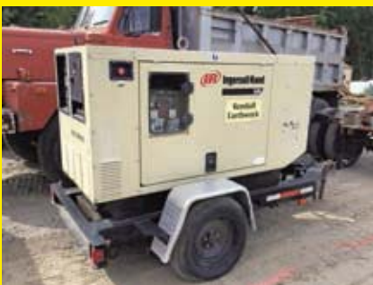
INGERSOLL RAND G40 Mitsubishi diesel engine, 40KW, 60HZ, 480V, trailer mounted.
