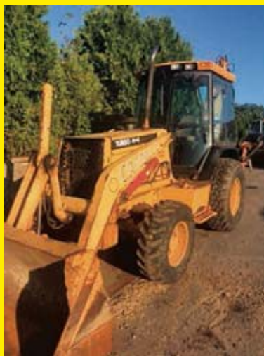
JOHN DEERE 310 SUPER E SN:T0310SE880164 4x4, John Deere diesel engine, EROPS, front & rear auxiliary hydraulics, tool circuit, extendahoe, GP front bucket, rear digging bucket.
