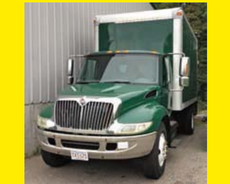
2003 INTERNATIONAL 4300 VN:591793 DT466 diesel engine, automatic transmission, power steering, 15ft. x 12ft. van body, power liftgate, dual wheel single axle.
