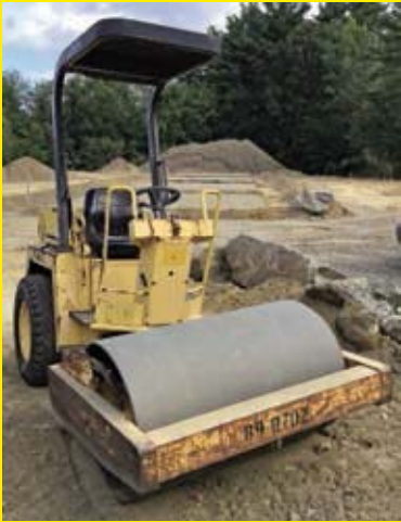
BOMAG BW124D Deutz diesel engine, EROPS, 48in. Smooth drum, vibratory drum, drum drive, 1,094 hours.
