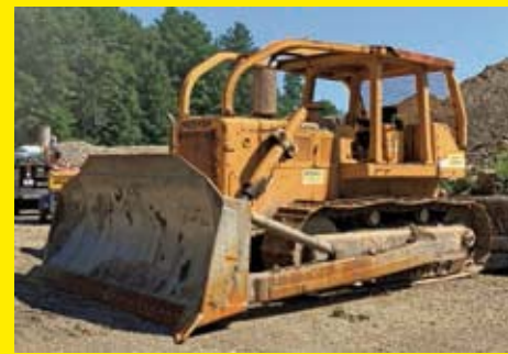
DRESSER TD25G International diesel engine, EROPS, 13ft. Blade w/ new cutting edge, 24in. Pads, low hours, original machine. HD Root Rake Sells Separately.
