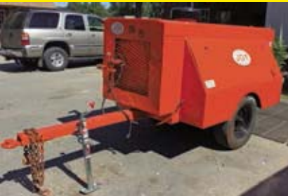
JOY 185 SN:162232 John Deere diesel engine, 185CFM, 2-new batteries, new starter & filter, hose & jackhammer, trailer mounted.
