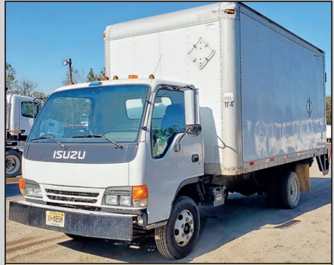
ISUZU NPR Box Truck with 2,000-Lb. Maxon Lift Gate, 14,500 GVWR, with 16' Morgan box, 38 cubic yard capacity.
