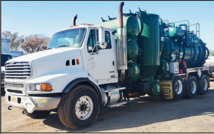
STERLING Tandem Axle L9500 Turbo Vac Truck , with 3,200-gallon capacity Presvac carbon turbo vac.
