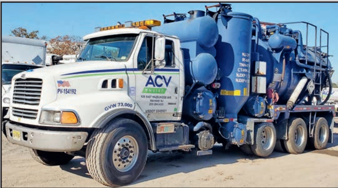
STERLING L951 Tag Axle Turbo Vac Truck , with 3,000-gallon capacity Presvac carbon high-dump turbo vac.
