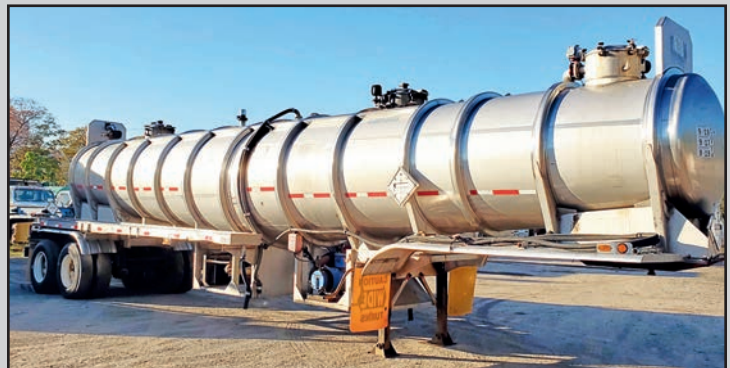
BRENNER Semi/Grey Vac Tank Trailer, 6,000-gallon capacity stainless steel tanker, with Fruitland 500LUF vac pump.
