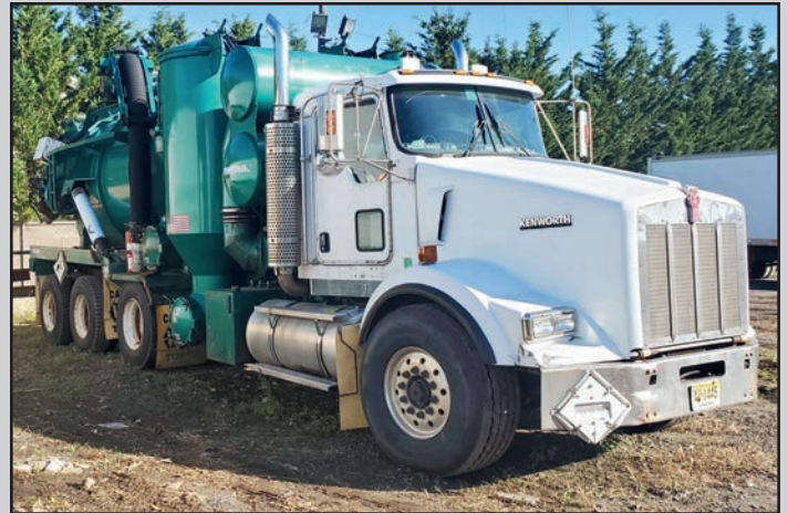
KENWORTH T800 Tag Axle Turbo Vac Truck , with 3,000-gallon capacity Presvac carbon high-dump turbo vac.
