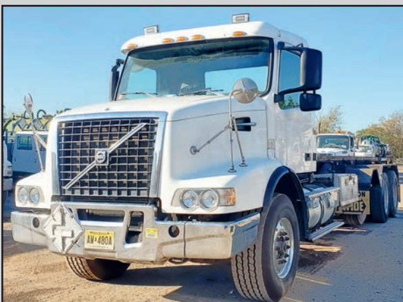
VOLVO VNT Roll-Off Truck, 20-30 cubic yard capacity.
