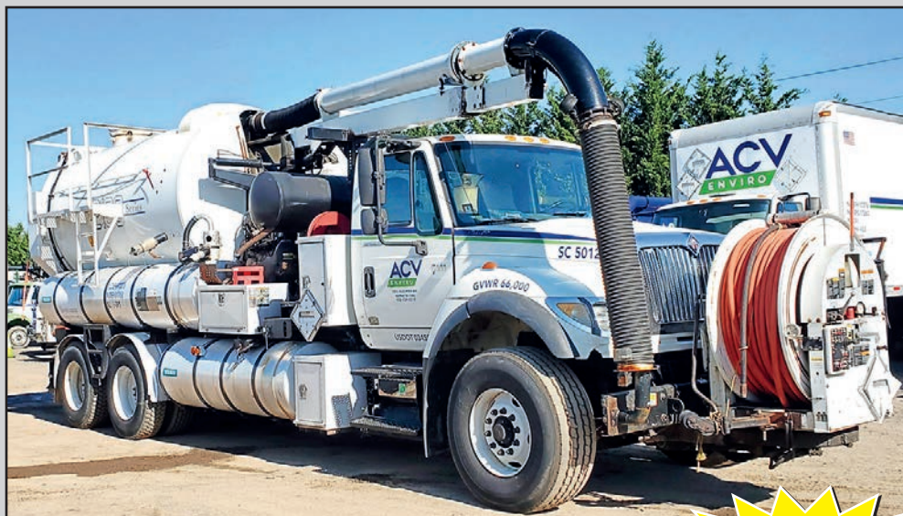
INTERNATIONAL Tandem Axle Sewer Cleaner Jet Rodder Truck, with 2,000-gallon capacity tank, 500' jetter hose.
