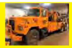
**1988 MACK DM6865X TRUCK** VN:1M2B128C6JA015528 Mack EM6 diesel engine, manual transmission, power steering, Holmes 1701 Lancer wrecker, 35 ton capacity, (2) 20 ton winches, camelback spring suspension, 12R24.5 tires, tandem axle, 95,085 miles.
