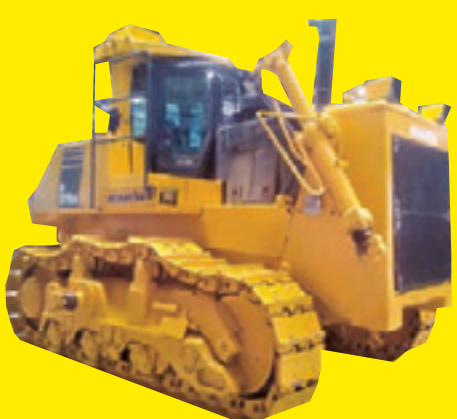
KOMATSU D375A-5 SN:18289 powered by Komatsu diesel engine, 515hp, equipped with EROPS, air, Straight blade w/ tilt, rear ripper.
