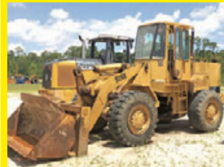
CAT 926E SN:94Z02283 powered by Cat diesel engine, equipped with EROPS, heat, quick coupler, GP bucket, 17.5 x 25 rubber. Forks Sell Separately.
