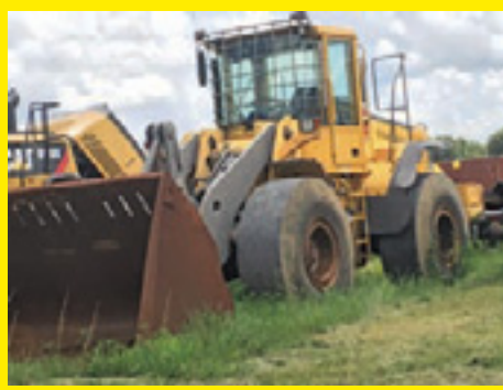
VOLVO L120E SN:EV64773 powered by diesel engine, equipped with EROPS, air, heat, GP bucket, solid rubber, 2,388 hours.
