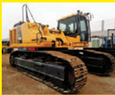
2011 KOMATSU PC600LC-8 SN:55277 powered by Komatsu diesel engine, equipped with Cab, air, reach boom, digging bucket, long undercarriage.
