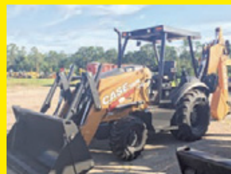
(2) UNUSED CASE 580N 4x4, powered by Case diesel engine, equipped with OROPS, powershuttle, extendahoe, switchable pilot controls, Case mechanical quick coupler, 4-in-1 front bucket, rear digging bucket.
