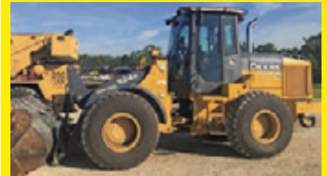
2015 JOHN DEERE 524K SN:JEE63526 powered by John Deere diesel engine, equipped with EROPS, air, quick coupler, GP bucket, 20.5 x 25 rubber.
