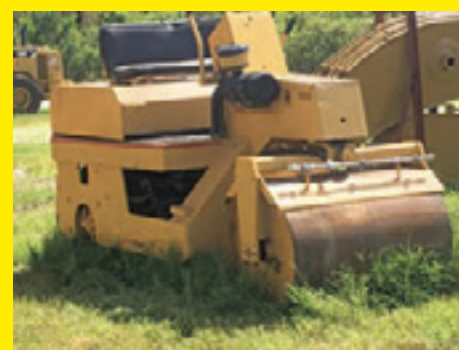
LEEBOY 400 SN:3769574 powered by diesel engine, equipped with 40in. Front smooth drum, 44in. Rear smooth drum.
