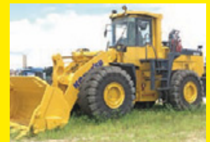
KOMATSU WA500 SN:52201 powered by Komatsu diesel engine, 315hp, equipped with EROPS, air, heat, GP bucket, 26.5 x 25 rubber.
