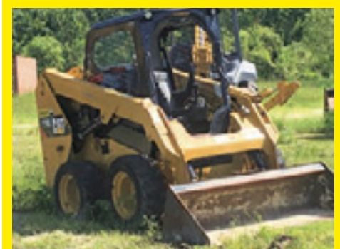
2014 CAT 236D SN:BGZ00904 powered by Cat diesel engine, equipped with rolldage, auxiliary hydraulics, mechanical quick coupler, GP bucket.
