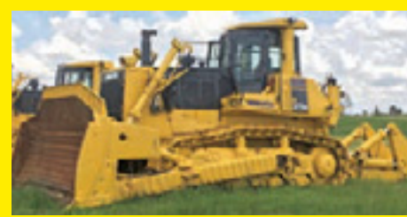
KOMATSU D375A-5 SN:18197 powered by Komatsu diesel engine, 515hp, equipped with EROPS, air, Straight blade w/ tilt, rear ripper.
