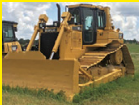
2007 CAT D6TLGP SN:KJL00477 powered by Cat diesel engine, equipped with EROPS, air, heat, Straight blade w/ hydraulic tilt.
