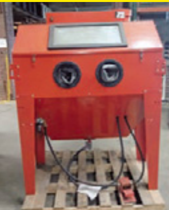
BLACK BULL SBC-420 SANDBLASTING CABINET 17 X 47IN. WORKING AREA
