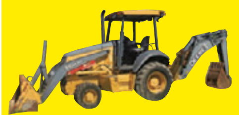
2014 JOHN DEERE 310K SN:260596 4x4, powered by John Deere 4.5L diesel engine, equipped with OROPS, pilot controls, 1.13 yard GP front bucket, rear digging bucket, Firestone 19.5L x 24, 12-16.5 tires, Extended Warranty (Comprehensive) 5000 hours or 12-26-19/ Extended Warranty 3000 hours or 12-28-19.
