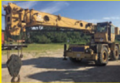
GROVE RT528E SN:68919 4x4, powered by diesel engine, equipped with Cab, 28 ton lift capacity, (4) hydraulic outriggers, rough terrain tires.
