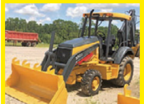
2011 JOHN DEERE 310J 4x4 SN:9587 powered by John Deere diesel engine, equipped with OROPS, rear auxiliary hydraulics, GP front bucket, rear digging bucket.
