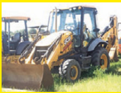
2012 JCB 3CX14 SN:2017623 4x4, powered by diesel engine, equipped with EROPS, air, extendahoe, front and rear auxiliary hydraulics, GP front bucket, rear digging bucket.
